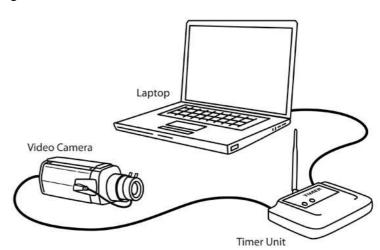
Connect the male power plug of the video/power cable (same end that is connected to the timer unit) to the 24 volt transformer. Plug in the transformer to a standard wall socket.
